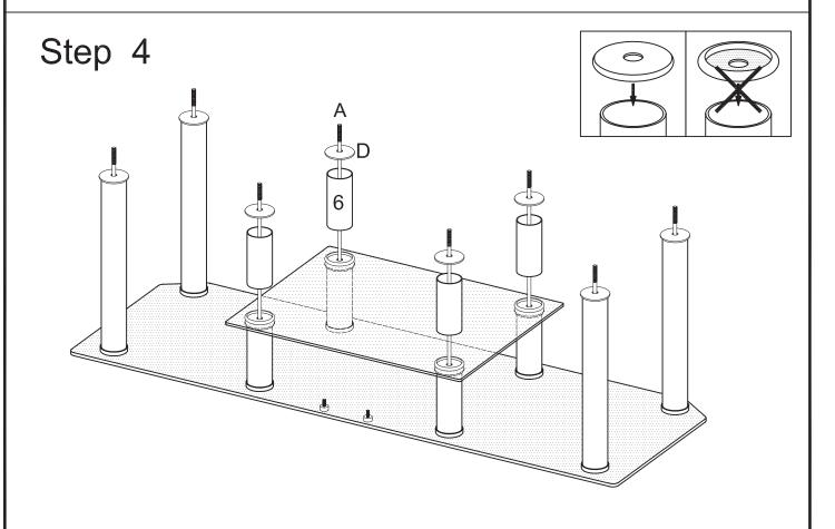
Slide cylinders (6) onto middle long rods (A). *Cylinders (6) will fit snuggly into the decorative rings placed in the previous step.* Slide decorative rings (D) onto middle long rods (A) and snap onto cylinders (6).
